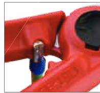
Special slot to crimp (0,5 - 4 mm 2 )
